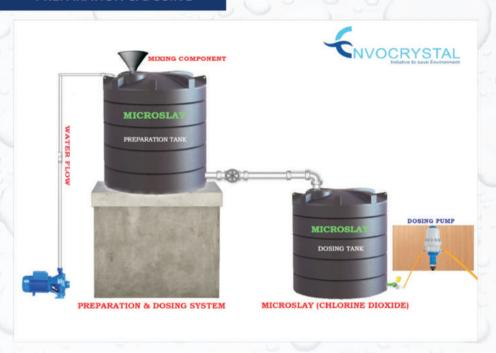
Take & fill the Tank with exact amount of tap water as shown on the label (1L, 5L, 10L, 50L. etc.) First add component A to water in Tank and then add component B. Securely close the tank. Wait for 4 hours for reaction to complete. After reaction MICROSLAY (CIO2) Solution is ready for use.
